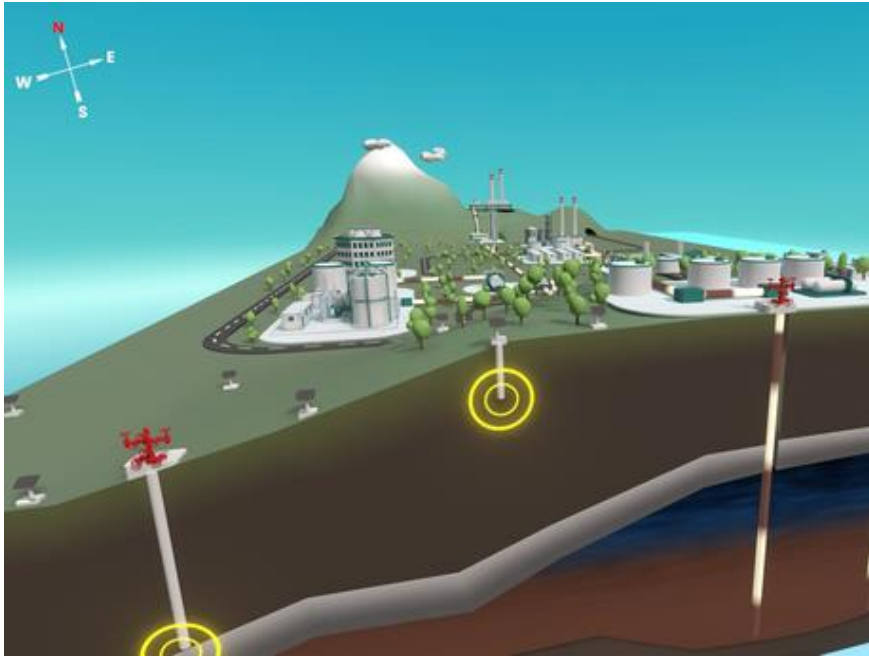
Figure 5: An example of a microseismic antenna that could operate in synergy with SpotLight focused seismic to target the same spot. The microseismic monitoring method is part of the CarbonWatch monitoring package for CCS, to which SpotLight focused monitoring has been added (source: www.bakerhughes.com ).
