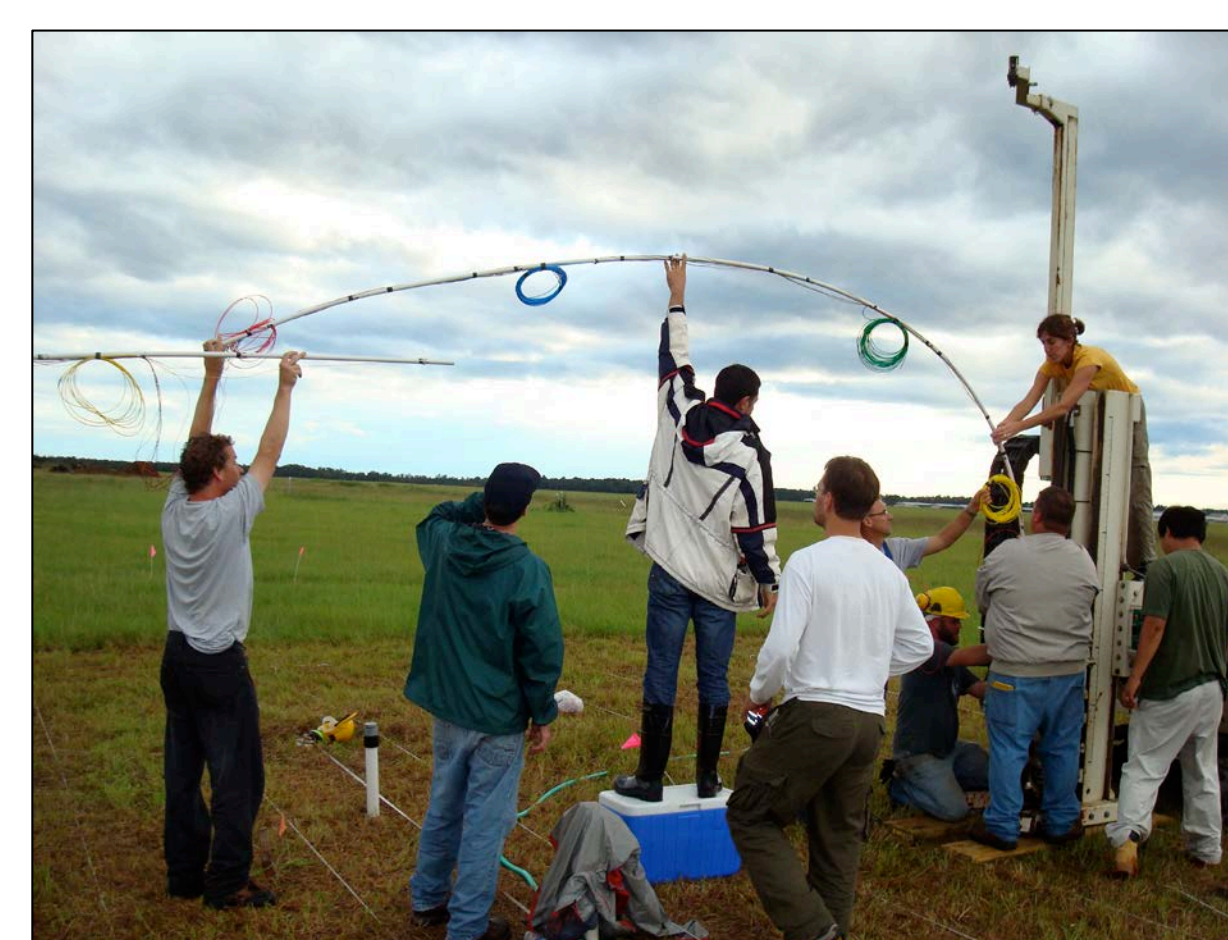
Installing multi-lever samplers
