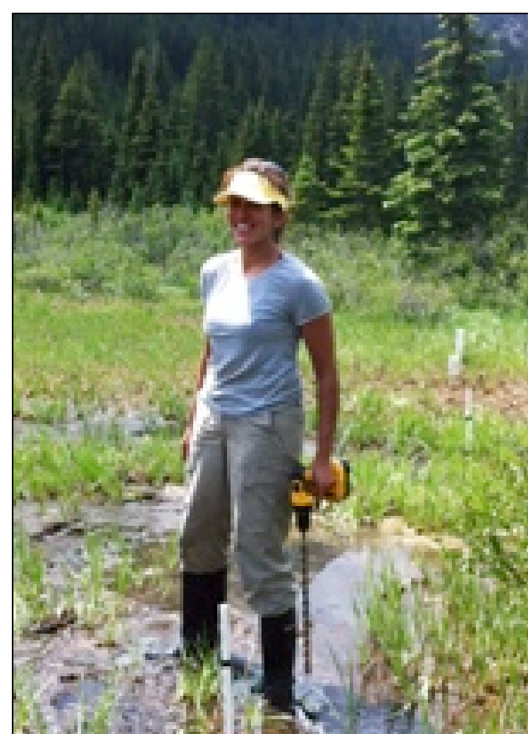
Drilling small piezometers
