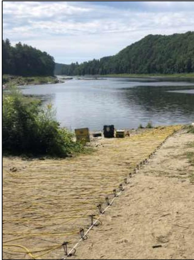
Electrical resistivity array installed along the edge of a water body.
