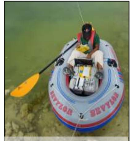
Tonian collecting a GPR profile over a sinkhole pool.
