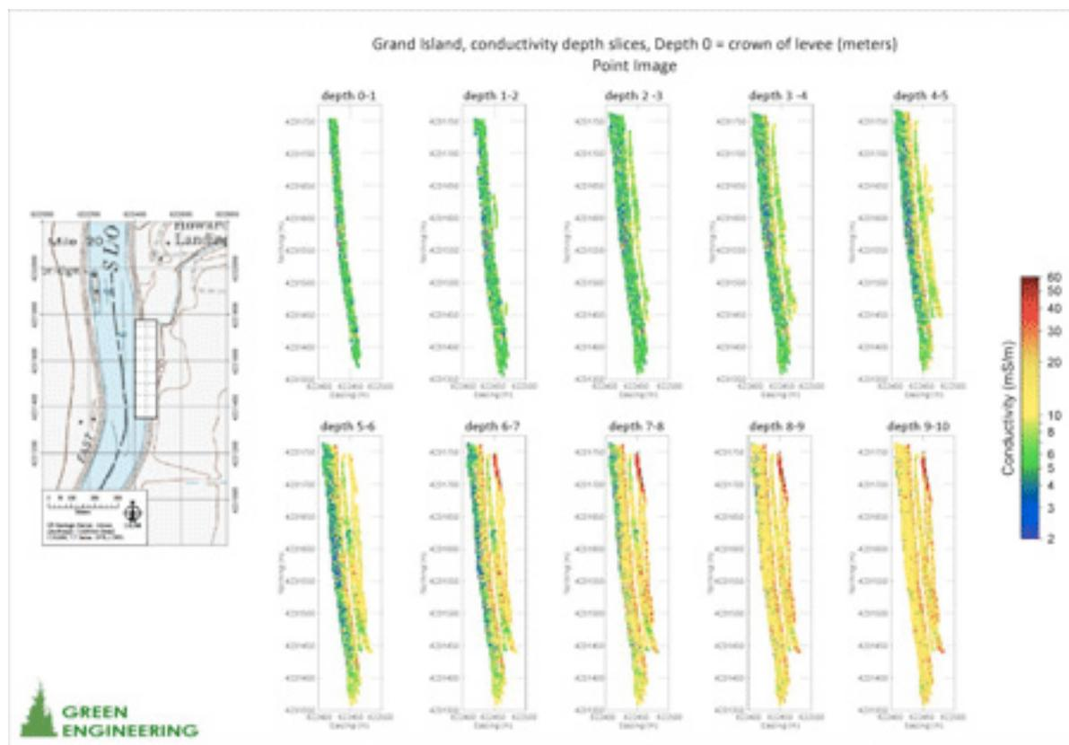
*Figure 7. Inverse models of a section of the Grand Island levee at 1 m depth slices. The location map is shown to the left. The model is presented as point images at an average sounding site.*
