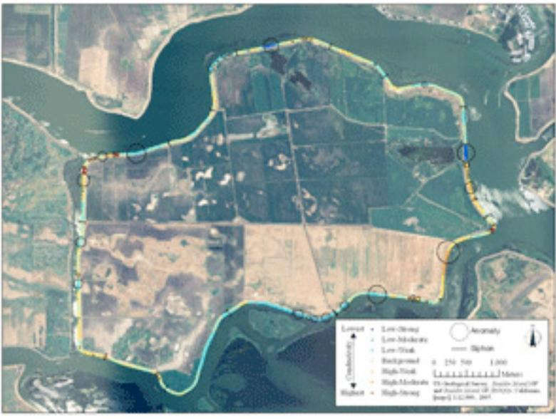
*Figure 3. Rapid scoping with low apparent conductivity (blue) at the sites of levee repairs, and high apparent conductivity in areas of finer texture and/or higher moisture content.*
