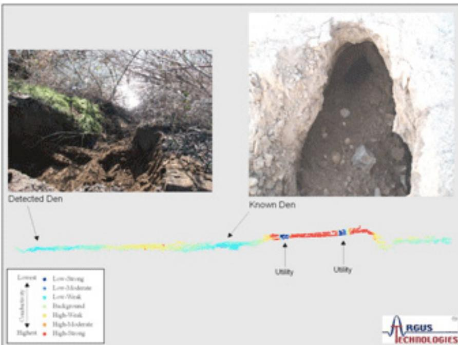
*Figure 6. A comprehensive characterization analysis resolved zones of low apparent conductivity that are associated with beaver dens.*
