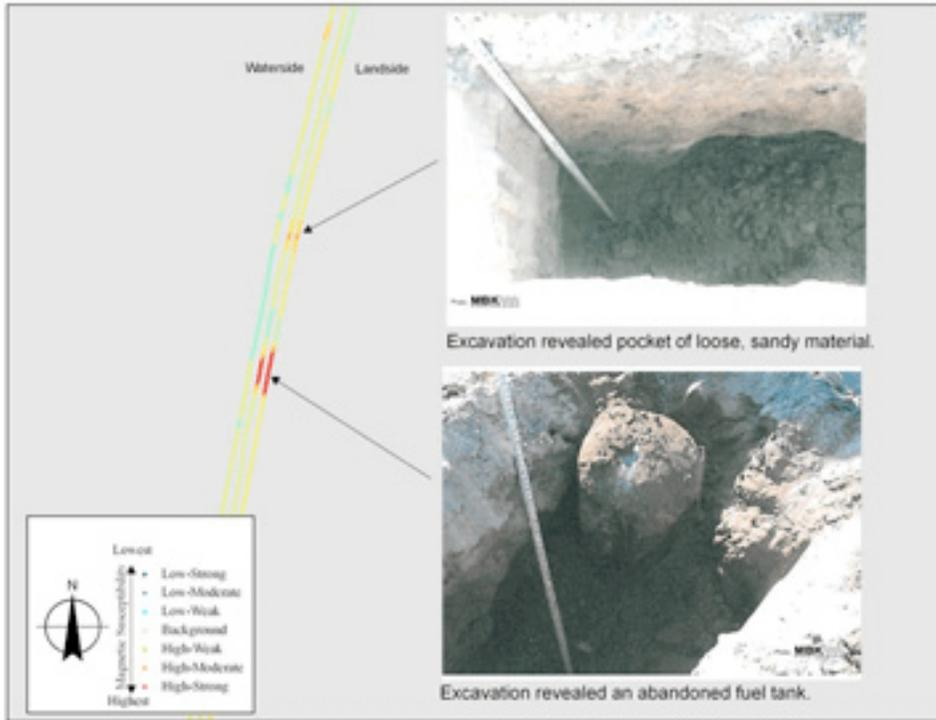
Figure 5. Based on the relative intensity of the anomaly, excavations are efficiently identified to the appropriate side of the levee.
