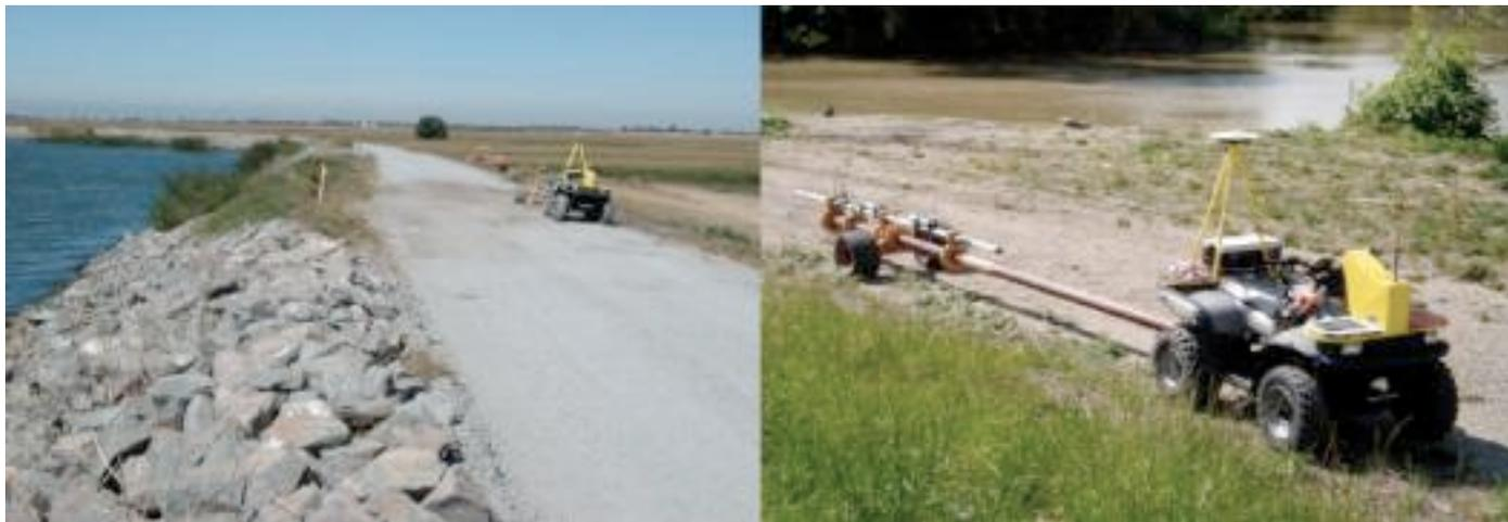
*Figure 2. The EM3 on-site for levee surveys.*
