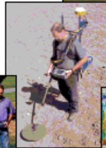
MetalMapper™ the first metal detector to work in magnetic soil.
