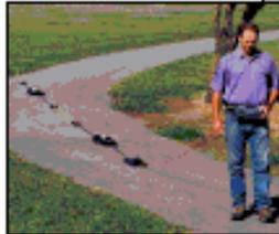
OhmMapper non-contact resistivity system. Fast, easy resistivity without stakes.
