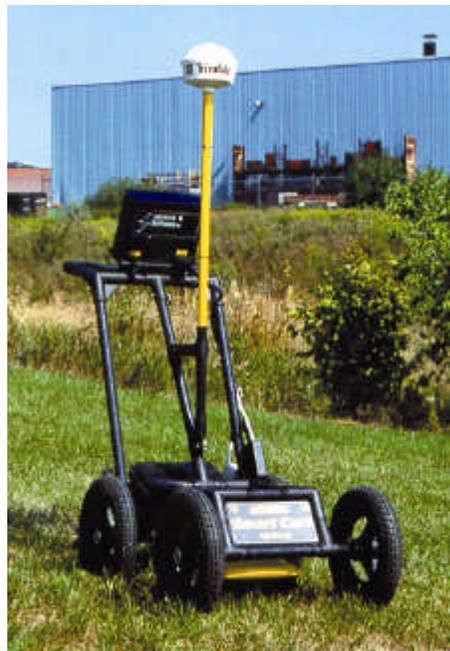
The Noggin family has rapidly expanded over the succeeding 4 years. The Noggin 500 and 1000 systems were introduced in quick succession along with the Noggin<sup>plus</sup> configurations. In addition, the Smart Cart and Smart Handle systems were developed to make GPR surveys simpler. In 2001, Conquest for concrete imaging and the Rock Noggin for rock and mine applications were introduced as the newest members of the Noggin family.
